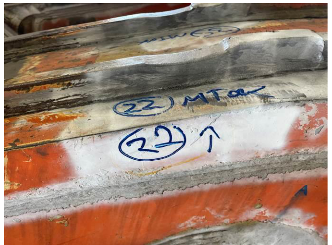
PHOTOGRAPH NO. 24 – EXTERNAL STICK TYPICAL VIEW OF REPAIRED DEFECT #24
