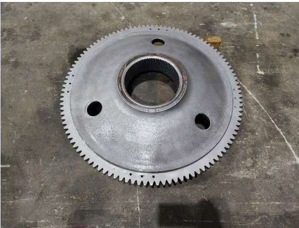
Photo 3 - Overview of Anchor Gear.
