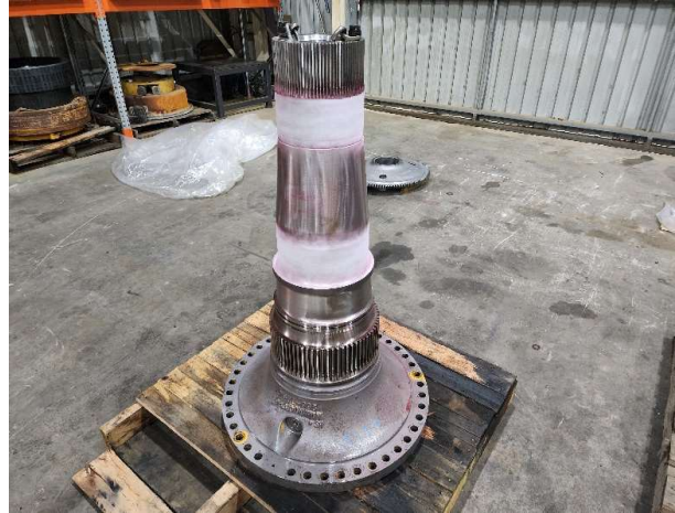
Photo 2 - Overview of Spindle inspected. Bearing journals sprayed white indicate extent of Dye Penetrant Testing.
