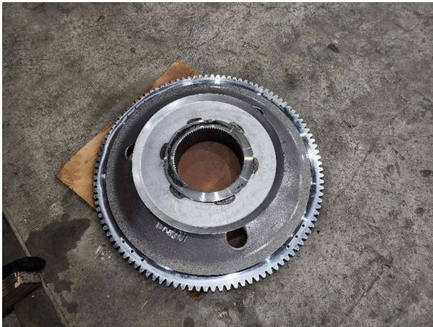
Photo 3 - Overview of Anchor Gear.
